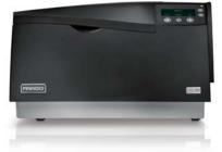
Versatility starts here. A basic DTC550 uses Fargo's Direct-to-Card technology to print full-color, single- and dualsided cards. Match specific needs with connectivity, lamination and e-card encoding options.
